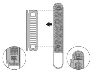
The bottom Mounting Knob thread in the hole and the top Mounting Knob sits at the groove.
